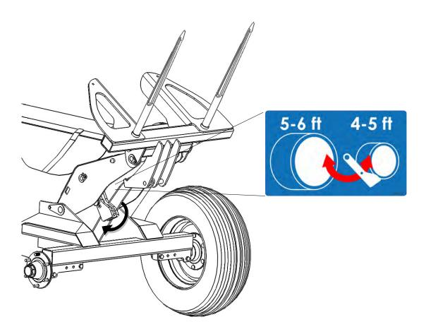
In order to set the G2x2 feeder up to load larger diameter round bales (5-6ft) it is necessary to lower the boom leg, to do this the boom must be in the fully raised position. Pull out the pin and rotate the leg down and lock it back into place. For loading smaller diameter bales, this leg must be folded back up
