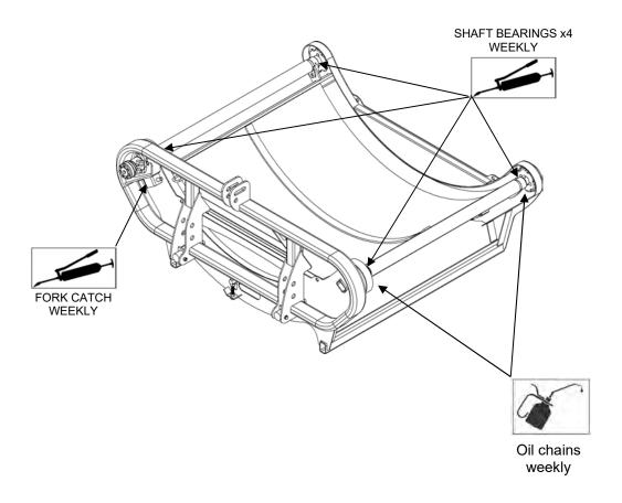
The feed chains should be lubricated on a weekly basis to prolong operational lifespan. Giltrap Engineering recommends the use of food grade chain oil to avoid contamination of livestock feed. To lubricate the chains the machine should be turned over at slow speed, and oil applied to the chains. Care must be taken to avoid contact with the machines moving parts.
