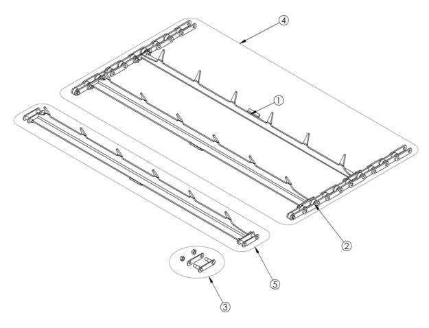
NOTE: If replacing bars on G2 bale feeder, item 5 must be used to guarantee correct compatibility
