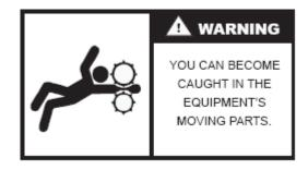
Wear proper protective clothing. Loose attire can easily be snagged by rotating machinery resulting in serious injury or death.
