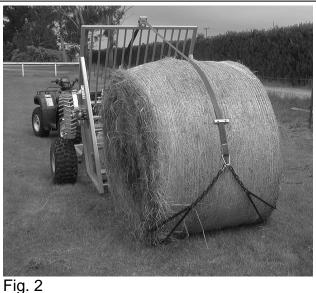
ensure the winch is locked with the ratchet (refer P10) to prevent the carriage from tipping backwards during transport or when the bale is fed out.
